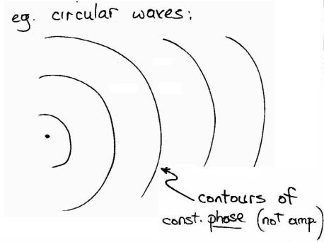
speed of propagation of point of fixed phase:  $X = \frac{1}{L}\phi + \frac{\omega}{L}t - \frac{1}{L}E$
