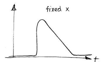
· wave maintains its shape for case considered here (n=const, indep. of frequency component re. "dispersionless").
